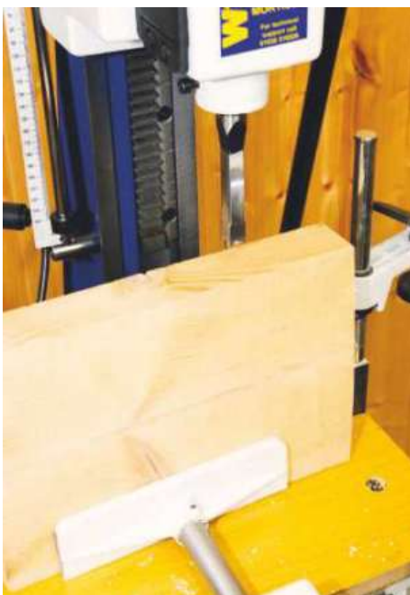
▲ Timber up to 205mm deep will fit below a 13mm chisel
